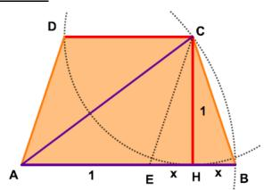
We draw segment CE, parallel to AD. Let us take the height of the trapezoid as 1. Then: AE = 1, AC = AB = 1 + 2x where x = EH = HB, and applying Pythagoras in  $\triangle$ AHC, rectangle in H:
